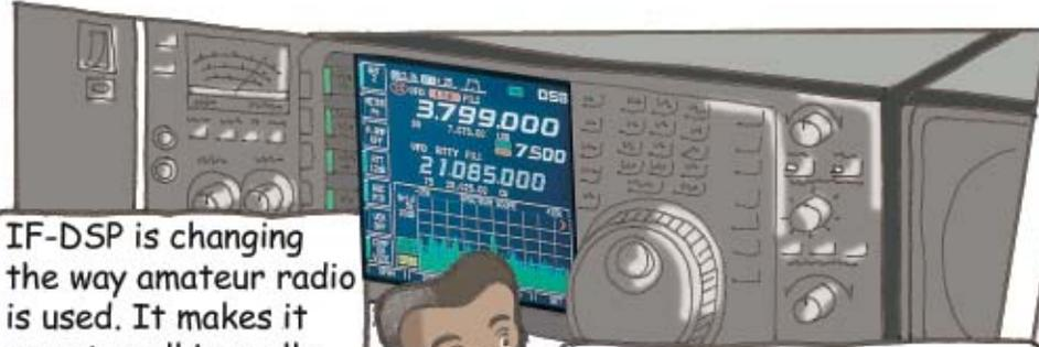
IF-DSP is changing the way amateur radio is used. It makes it easy to pull in really far away stations or to isolate a single signal, like you're hearing today.
